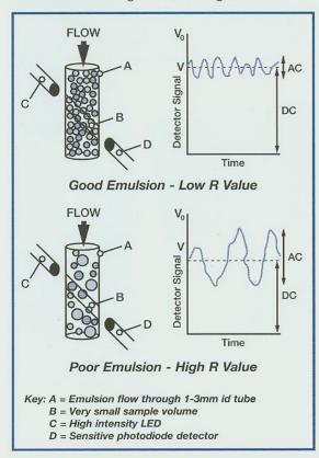
illuminates the flowing emulsion and the transmitted light is monitored by a sensitive detector, which produces a signal comprising two components:
