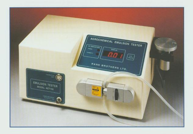
The Model AET100 is a simple, rugged instrument designed to test the stability of water-based agrochemical emulsions which are widely used in pest control. Easily surpassing the performance of earlier methods, the turbidity fluctuation analysis technique can quickly and precisely characterise emulsions to bring significant benefits to testing in the development of new formulations and the quality of manufactured emulsifiable concentrate products.
