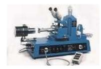
The **Photometric Dispersion Analyser** (**PDA2000**) is a simple, rugged, but very sensitive monitor for flowing suspensions and emulsions, based on an optical technique developed at the *University College London*.
