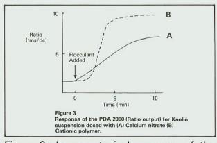
Figure 3 shows a typical response of the PDA 2000 used in this way. The suspension is of clay (kaolin) and the additives are a calcium salt and a cationic
