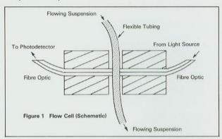
When aggregation of particles occurs, the rms value of the fluctuating signal increases (ref. 1). Measurable changes in the rms value occur long before any visible signs of aggregation are apparent. Conversely, when aggregates are disrupted, the rms value decreases, reaching a minimum when disaggregation (or dispersion) is complete. The dc value (related to the turbidity) is much less sensitive to changes in the state of aggregation.
