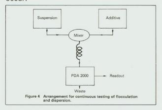
Tube flow is a very convenient basis for a laboratory flocculation test and the PDA 2000 is an ideal monitor for such applications. Changes in flocculant dosage cause a corresponding change in the ratio output after an interval which depends on the residence time in the tube.
