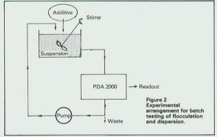
After passing through the flow cell the sample can be returned to the vessel by means of a peristaltic pump or can go to waste. A range of different dosages of additive (dispersant or flocculant) can be explored and the response of the PDA 2000 (usually the ratio output) can be monitored. The speed of response depends on the suspension concentration—from as little as a few seconds for concentrated
