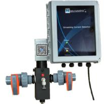
The Streaming Current Detector / Transmitter Model SCD-T is designed to be used with the Water Treatment Controller Model W610. It is also compatible with Process Controllers/Analyzers, PLCs, and SCADA. The Model SCD-T includes an integral streaming current sensor and electronics transmitter. Streaming Current Detectors have demonstrated the ability to optimize coagulant dosing and prevent plant upsets.
